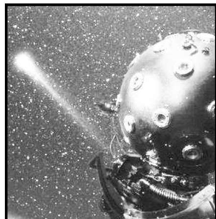
The Korkosz Projektor Korkosz Projector in Springfield, 1937: The first projector not manufactured by Zeiss was constructed by the brothers Frank and John Korkosz in Springfield, Massachusetts. It was a sphere of one meter and displayed 7150 stars down to the 5 th magnitude but no planets. The star fields were arranged on 41 individual plates.
